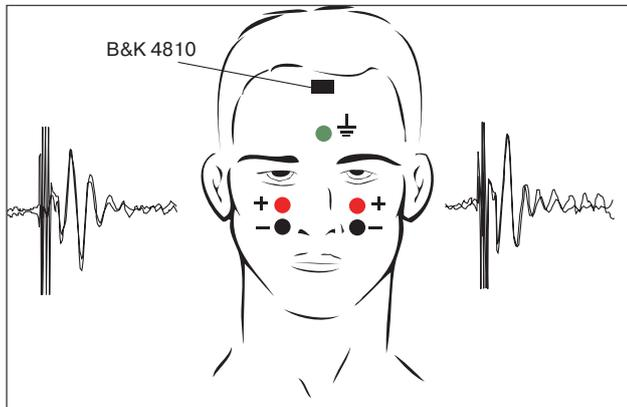
Fig. 10. BC oVEMP: electrodes and responses
