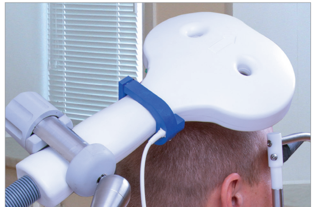
Tracking sensor on TMS coil
